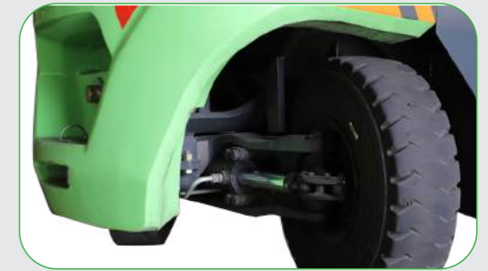
Steering Axle • Enlarging the steering axle angle, thickening the oil cylinder and replacing ordinary bearings with tapered roller bearings, so as to achieve high reliability, small turning radius and less tire wear
