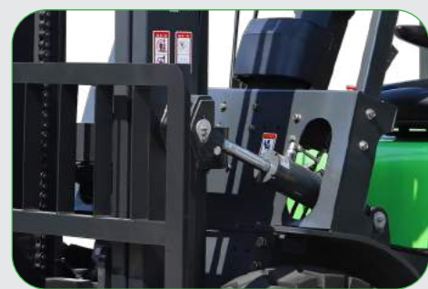
High Fulcrum Tilt Cylinder Mounting • The high fulcrum design of the tilt cylinder mounting makes the mast more stable and reliable
