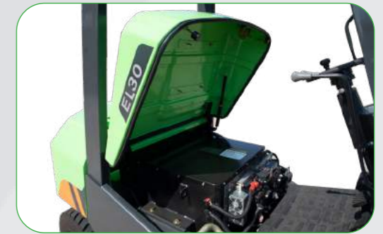
Large Angle Opening of Engine Hood • The opening angle of the hood is large, and the battery, electric control, and motor can be accessed directly after opening the hood, which makes maintenance more convenient Removing Floor with Tool-free • Simple operation, saving time and labor for routine maintenance
