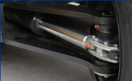
02 Heavy duty steering axle with tapered bearings.
