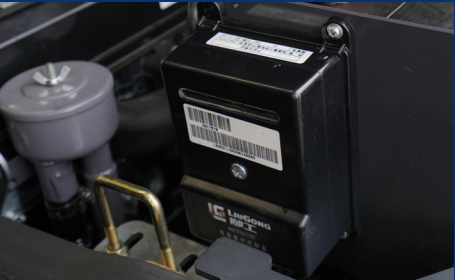
01 The integrated electric box makes maintenance and repair convenient with better water-proof performance.
